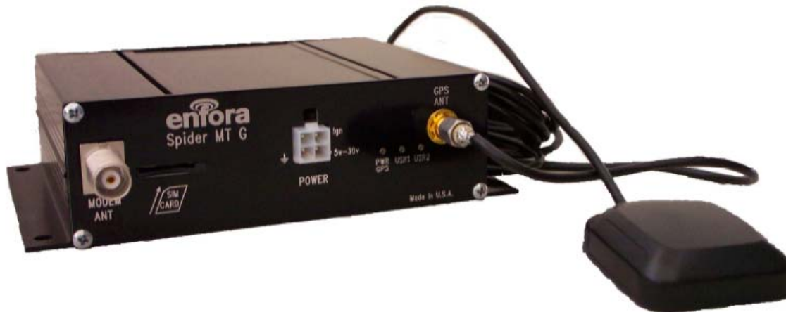
Figure 9 - GPS Antenna Connection
