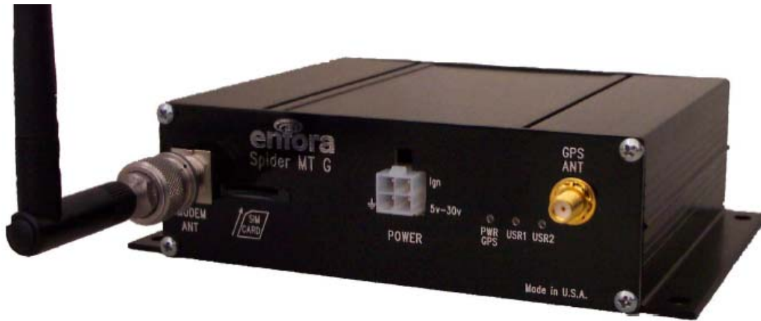
Figure 8 - GSM Antenna Connection
